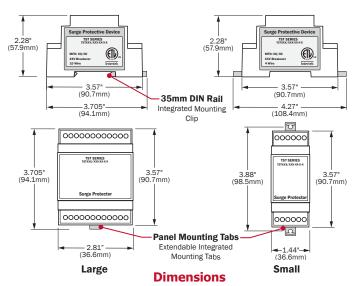
The TST Series of SPDs (surge protection devices) are designed to protect sensitive electronic equipment from the harmful effects of transients.
