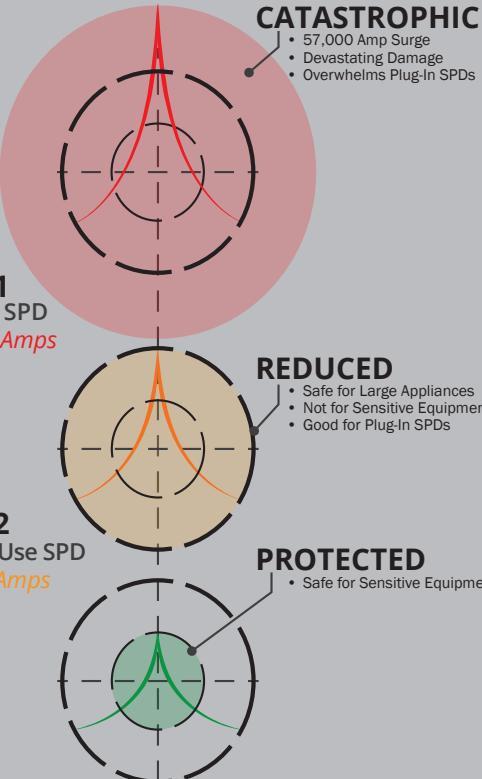
By **diverting over 95% of the Surge Energy to ground** before the Surge enters your home, the remaining energy is now **within the typical capacity of a plug-in Surge Protector** and Uninterrupted Power Supply (a.k.a. battery backup with surge protection) which protects your most sensitive equipment. **SPDs for generators and solar panels** may also be required (covering other "service entrances" to your home).
