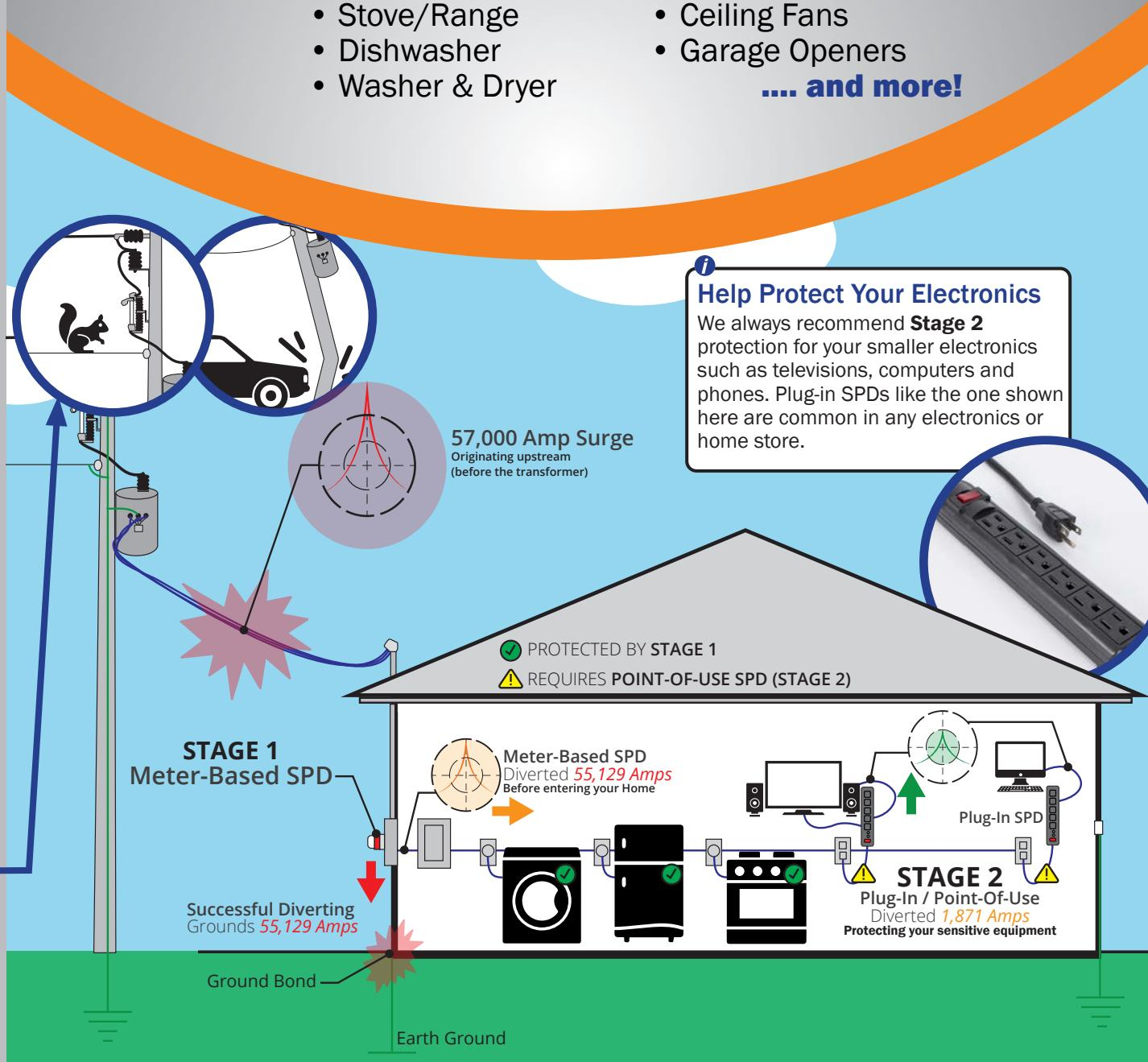
This diagram shows how your new surge protection device will work to help protect your home against electrical surges. When a surge enters the home through the meter, **your surge protection device will block** (shorting to ground) the **excessive voltage** that is not safe for your large appliances.
