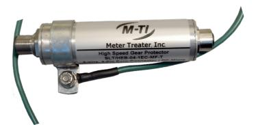
The SLT High Speed Gear Sensor Protector is 5 Wire SPD (surge protective device) unit that will interface directly, in series, with 5 pin M12/Euro/DC Micro Connectors. Unit is unidirectional due to connector configuration; where the male connector equals Line Side (unprotected) and the female equals the Load Side (protected). Circuit performance is bidirectional.
